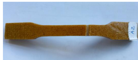
Figure 8. Broken tensile test piece
