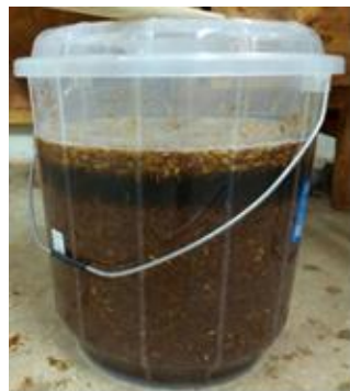
Figure 2. Rice husks immersed in 4% NaOH
