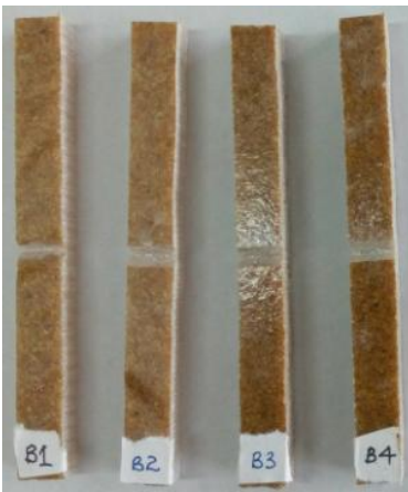
Figure 5. Impact test specimen samples
