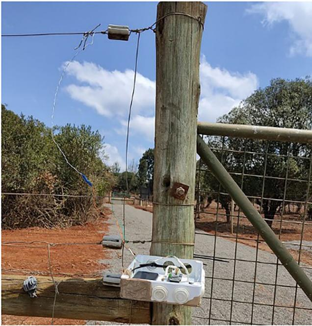
**FIGURE 21** The Raspberry Pi time domain reflectometer connected to the electric fence at the Dedan Kimathi University of Technology Wildlife Conservancy.
