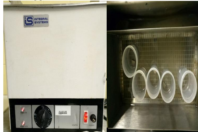
Fig. 16. Sample Preparation: Ultrasonic cleaning process
