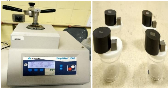
Fig. 14. Sample Preparation: Mounting process
