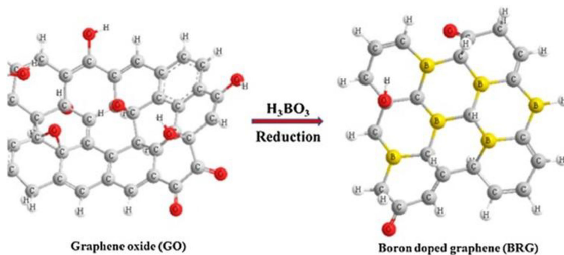
Figure 6. The formation of boron-doped graphene (BRG) from graphene oxide (GO). Adapted with permission. [87] Copyright 2018, Elsevier.
