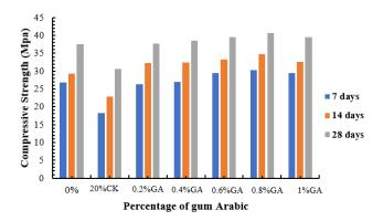
Fig. 10 Compressive strength with CK and GAB content
