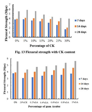
Fig. 14 Flexural strength with GAB and CK content
