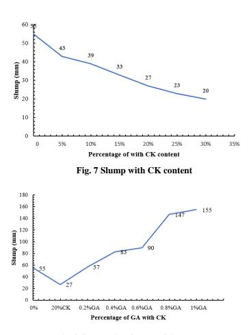
Fig. 8 Slump with CK and GAB content
