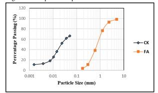
Fig. 1 Calcined Kaolin and fine aggrate distribution curve
