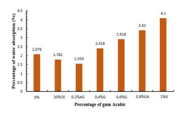
Fig. 6 Water absorption with CK and GA content
