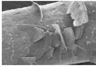
Fig. 3: SEM micrograph of hair shaft showing initial stages of surface degradation, (mag. x1.0K, 5.0kV).
