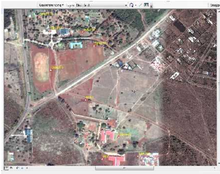
Figure 6 Georeferencing aerial photo using new geodetic control points at DeKUT
