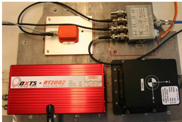
Figure 1: Overview of Applanix IMU (lower right), OXTS (lower left), Xsens MTi-G (upper left) and GPS power splitter
