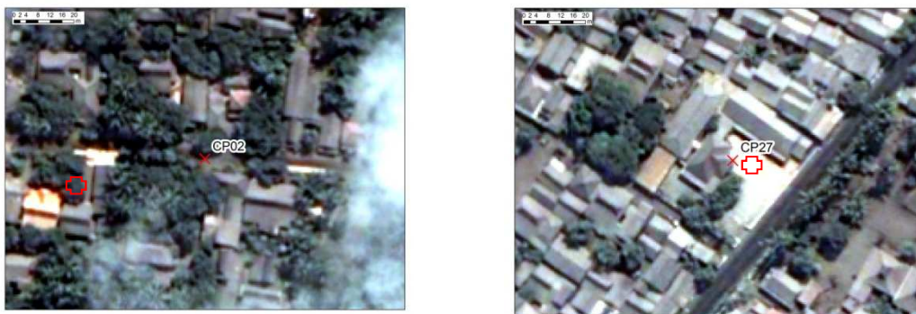
Figure 3: Blunder error detection (+: before orthorectification, x: after orthorectification)
