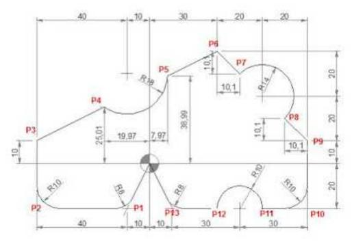
b) Prepare a CNC part program to mill the component represented in the following drawing. [10 Marks]
