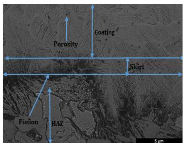
Fig. 5. Porosity in the sample coated at 60 A DC. The optical microscopic image was taken along the coating-substrate cross-section.
