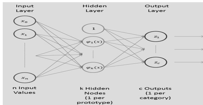
Fig. 6: Typical architecture of an RBF Network.
