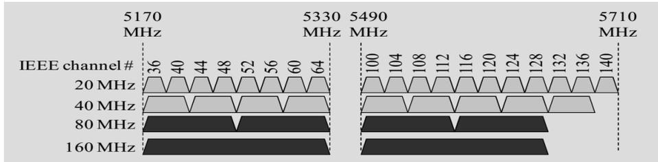
Fig. 4: Europe and Japan Bandwidth and channel allocation.
