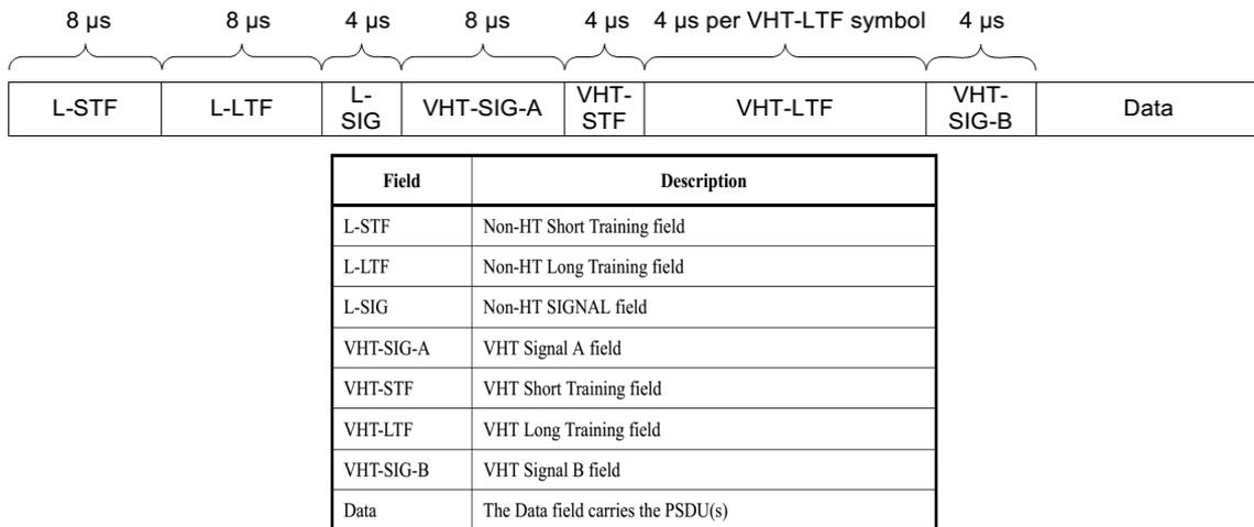
Fig. 2: IEEE 802.11 packet structure and timing related constants
