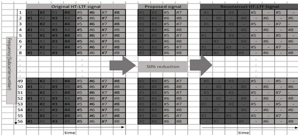
Fig. 5: Proposed system with 1/2 VHT-LTF preamble
