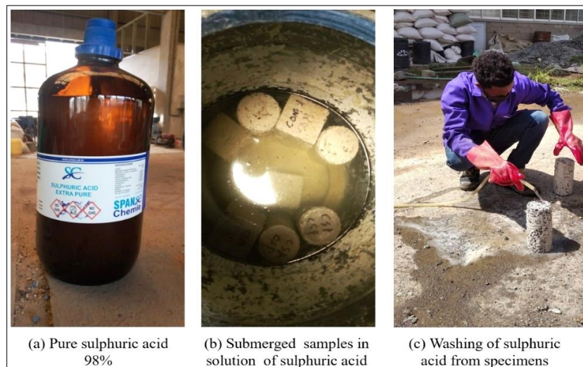
Figure 8. Conducting durability test for concrete samples exposed to sulphuric acid
