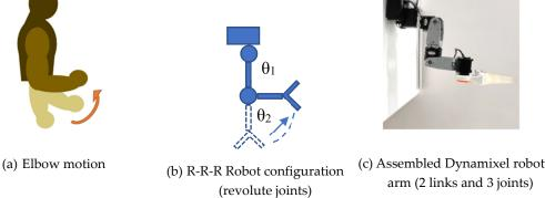
Figure 3. Robot arm configuration.
