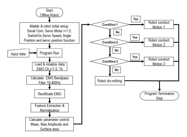
Figure 2. Flow chart offline robot control.
