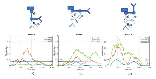
**Figure 9.** Upper pictures for subfigure (**a**–**c**) are shown each robot arm motions, besides lower pictures show discrimination of the EMG signal motion 1, motion 2, and motion 3 respectively.
