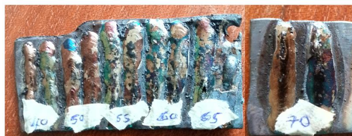
Figure 1: Stainless steel coated mild steel samples at different DC currents
