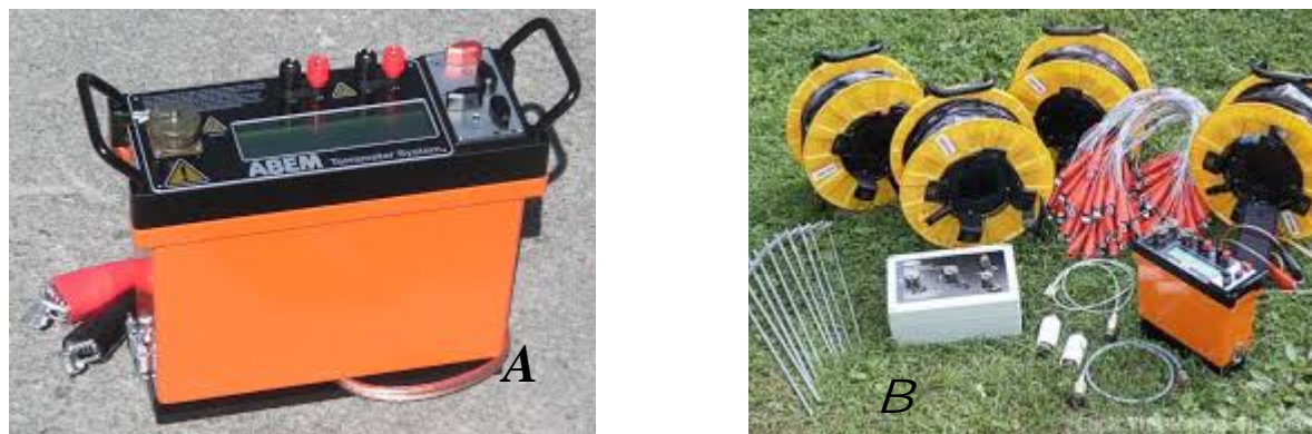
Figure 3.1: SAS 4000 Terrameter instrument used to collect and record the electrical resistivity data. B, electrodes and cable attachment used for electrical resistivity profiling
