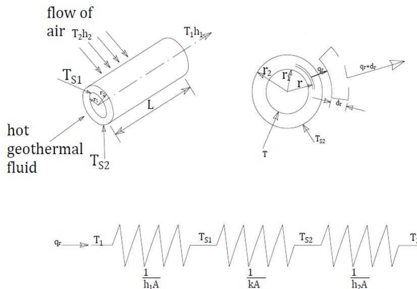
**Figure 1:** Heat transfer across the heat exchanger pipes (Adopted and modified from Incropera, 2005)
