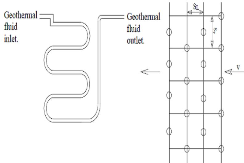
Figure 2: Heat exchanger pipes layout (Adopted and modified from Incropera, 2005)
