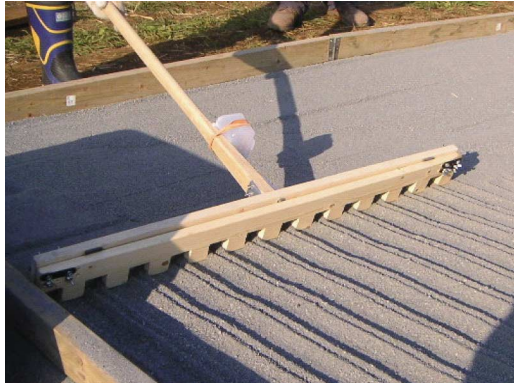
Fig. 3. Generation of a 4-cm roughness pattern using the roughness tool.
